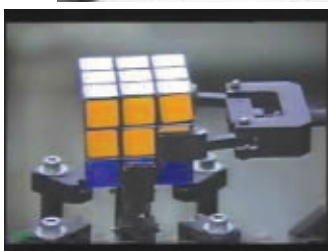
Figure 13. The Battelle Cubot's two Rubik's Cube grippers.
