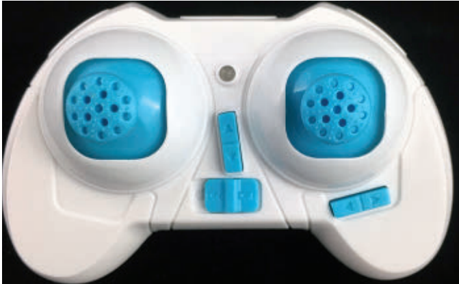
Figure 5: The remote is very simple, with two joysticks, trim controls, and a power switch. Each joystick is also a button, with the left changing the controller sensitivity and the right enabling the flip trick.
