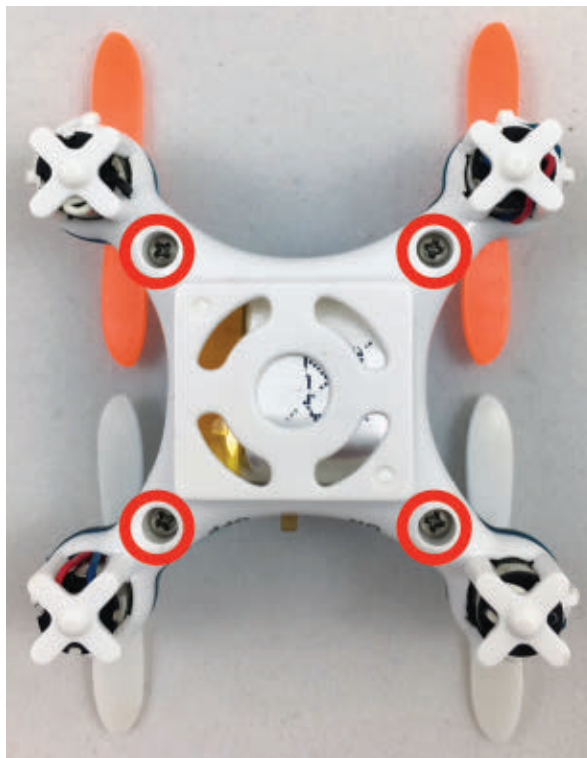
Figure 4: Removing four small Phillips screws is all it takes to pull apart the halves of the copter.
