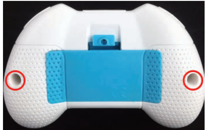
Figure 6: Remove the two screws in the back of the controller to separate the halves. Some controllers seem to have a third screw holding the battery door on, but it is not necessary to remove this screw to take apart the controller.
