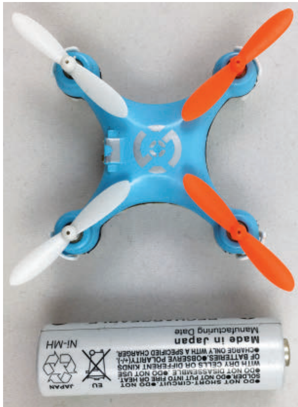
Figure 3: The CX-10 has a propeller center spacing less than the length of an AA battery. After-market propellers are available in many colors to make it easier to distinguish the orientation of the quad, and differentiate between multiple quads in flight.
